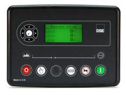
The DSE6110 MKIII is an Auto Start Control Module suitable for a wide variety of single, diesel or gas, genset applications. Monitoring an extensive number of engine parameters, the module will display warnings, shutdown and engine status information on the back-lit LCD screen, illuminated LEDs and remote PC.
